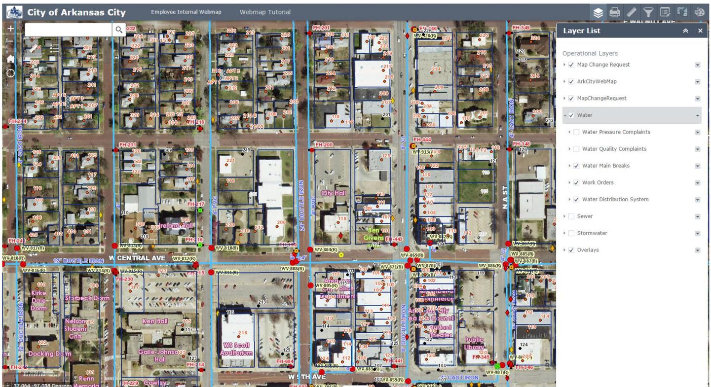
This works the same way for Sewer and Stormwater systems. The Overlays layer contains layers that are overlaid with transparency on the map. This includes layers such as zoning districts, floodplains, sanitation pickup days and similar layers. Clicking the various checkboxes there will turn them off and on.
